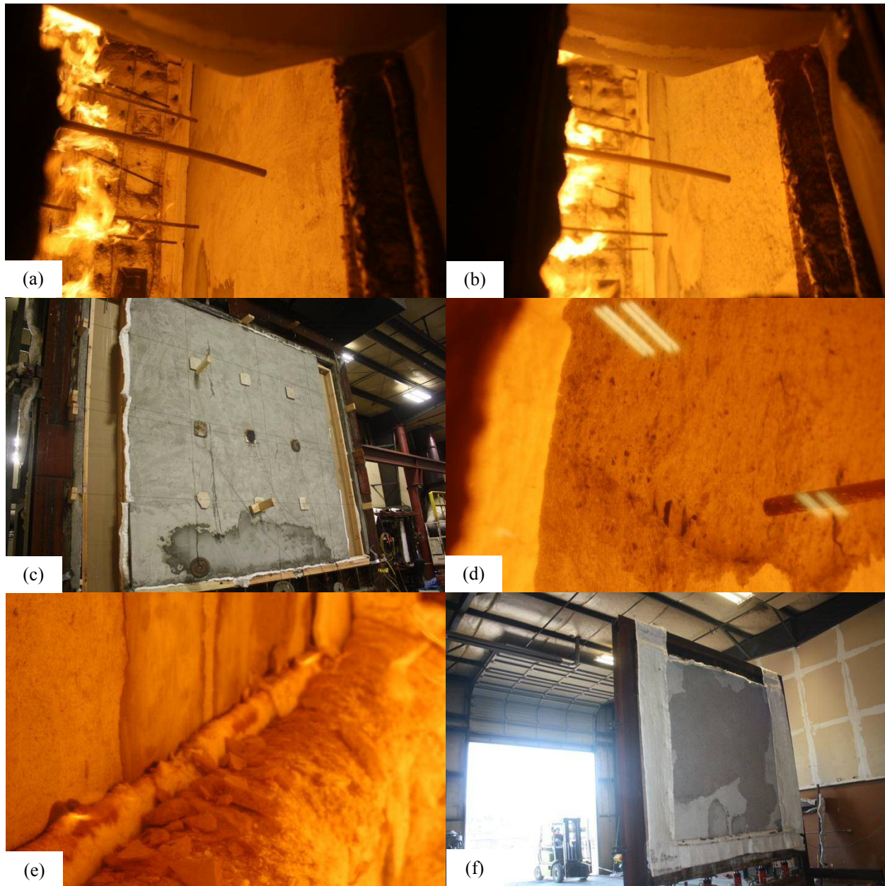
Figure 3. Wall assembly during fire resistance test showing (a) beginning of test – 2 min, (b) spalled face – 16 min, (c) dripping water – 27 min, (d) surface hole – 34 min, (e) bottom flaming – 44 min, and (f) assembly following test.
