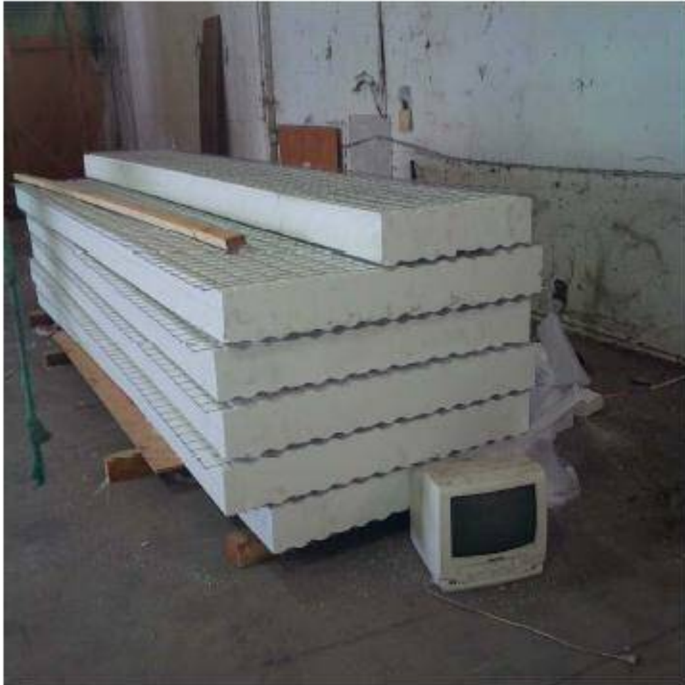
Photo 1. Schnell EPS / Wire Mesh Panels Used in Test Wall Assembly
